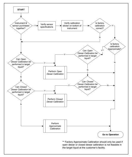
Figure 3-2. Calibration method selection diagram.
