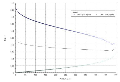
*Figure 2-1.* Dielectric vs. pressure for nitrogen under saturated conditions. (The center line indicates the discrimination point for immersed or exposed indication.)
