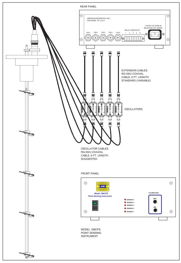
Model 188CPS Point-Sensing System Diagram (not drawn to scale).
