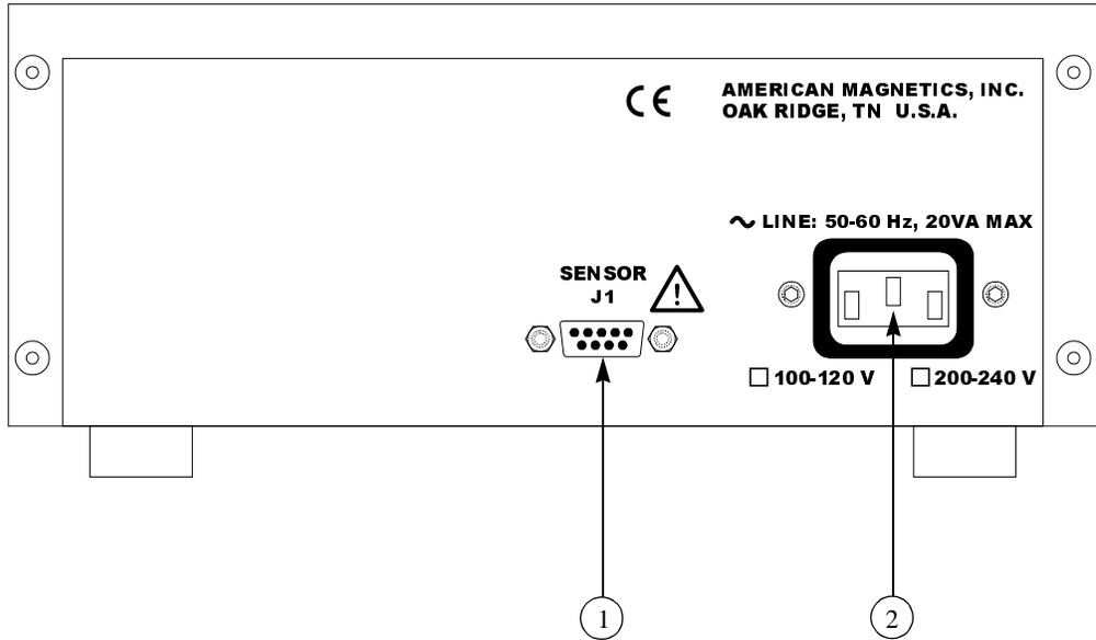
**1** Sensor input/analog outputs DB-9 female connector (see the *Appendix* for the pinout diagram)
