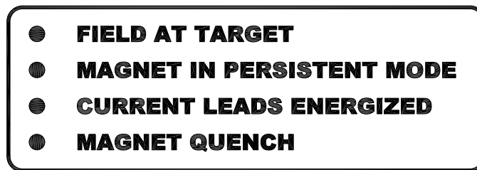
Figure 3-6. Magnet Status LED Indicators.
