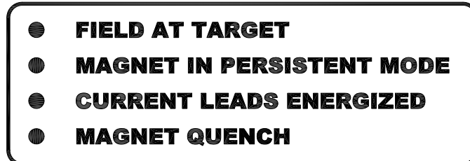
Figure 3-6. Magnet Status LED Indicators.
