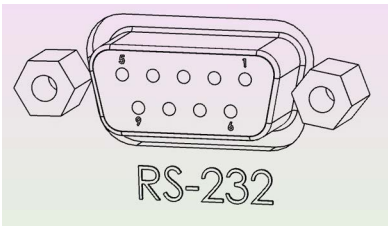
Serial (RS-232) Pin Out
