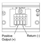
Figure 2.7-4 Output Voltage Connector (For high voltage models.)
