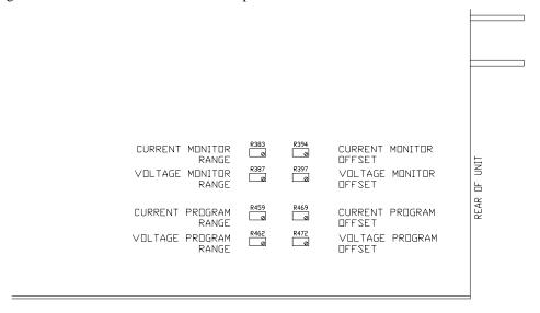
Figure 5.2-1 Programming and Monitoring Calibration Locations (Top view.)
