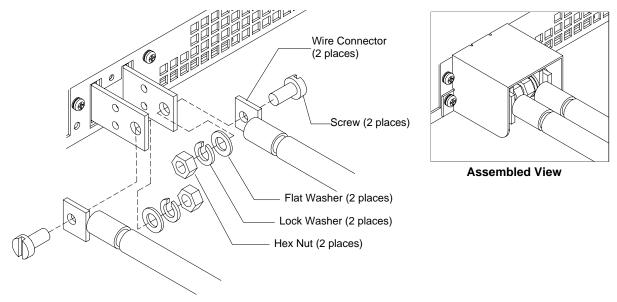
Figure 2.7-3 Typical Load Connection Hardware (Low voltage model shown.)
