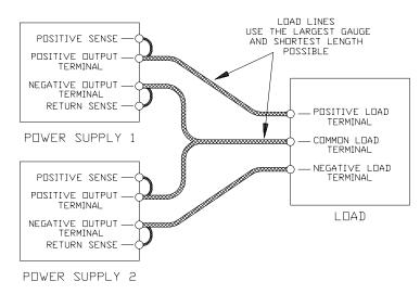
Figure 3.5-4 Split Supply Operation of Multiple Supplies (Positive-negative Supply)
