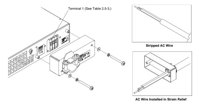
Figure 2.5-1 AC Input Cover and Strain Relief
