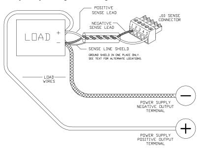
Figure 2.8-2 Connecting Remote Sense Lines
