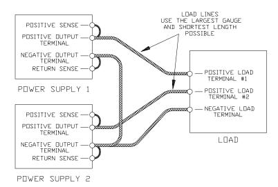
Figure 3.5-3 Split Supply Operation of Multiple Supplies (Two Positive Voltages)
