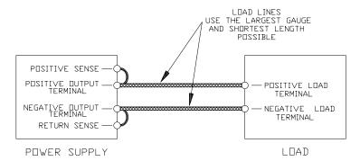
Figure 2.7-5 Single Load with Local Sensing (Default)
