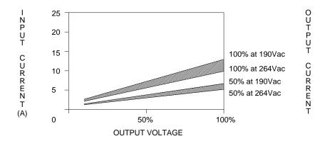
Figure 1.3-2 Typical Input Current Characteristics, 190-264Vac Range (Based on 60V, 20A model.)
