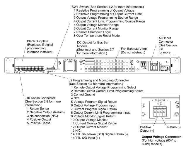
**Figure 2.3-2 Power Supply Rear Panel** (Low voltage (7.5V to 40V) model shown.)
