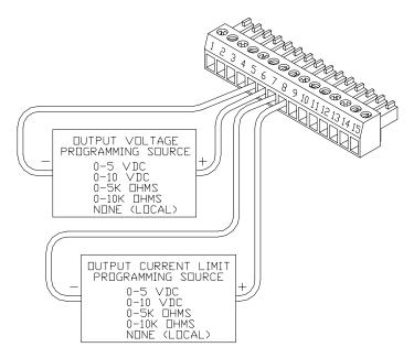
Figure 4.3-1 Connecting Programming Sources to J2 Connector
