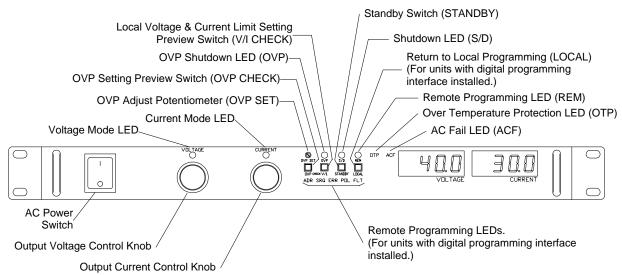
Figure 2.3-1 Power Supply Front Panel
