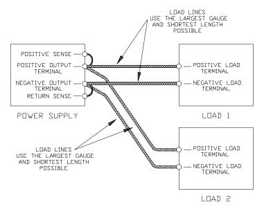
Figure 2.7-7 Multiple Loads with Local Sensing
