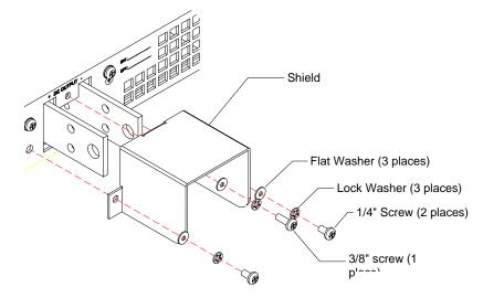
Figure 2.7-2 Bus Bar Shield
