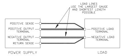
Figure 2.7-6 Single Load with Remote Sensing
