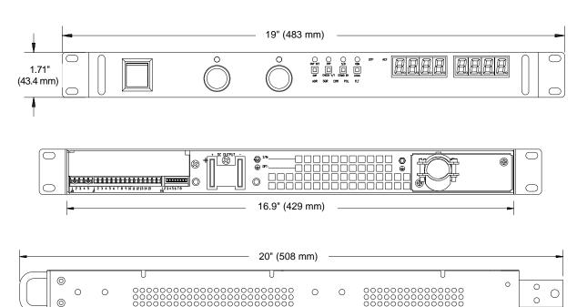
Figure 1.3-3 Dimensional Drawings (Dimensions given are nominal.)
