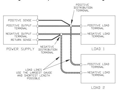
Figure 2.7-8 Multiple Loads with Remote Sensing
