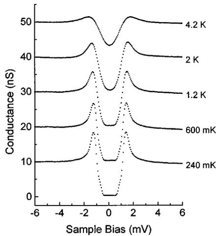
FIG. 5. Set of  $dI/dV$  curves measured with lock-in amplifier on the same sample as in Fig. 4 at various temperatures. (Modulation frequency  $f_{\text{mod}} = 331$  Hz, amplitude  $A_{\text{mod}}$  is  $40 \mu\text{V}_{\text{rms}}$  for the curve at 240 mK and  $80 \mu\text{V}_{\text{rms}}$  for the rest, 288 data points in 20 min acquisition time for each curve.) The curves are offset for clear display. The temperature dependence of the superconducting energy gap is well resolved.
