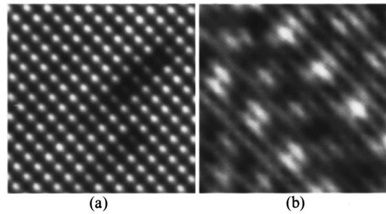
FIG. 7. Images of two surfaces which were exposed after cleavage of single crystal YBCO. (a) BaO plane ( $I = 1$  nA,  $V_{\text{sample}} = 100$  mV) with clear atomic resolution and several defects (darker sites). (b) CuO chain plane ( $I = 30$  pA,  $V_{\text{sample}} = 60$  mV), showing atomic resolution overlaid with a strong DOS modulation. Both images are  $50 \text{ \AA}$  square.
