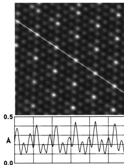
FIG. 4. Constant current image on NbSe<sub>2</sub> at 240 mK. ( $I = 50$  pA,  $V_{\text{sample}} = -50$  mV,  $50 \text{ \AA}$  scan range) below the image a line-profile position marked on the image shows the apparent atomic corrugation and CDW modulation.
