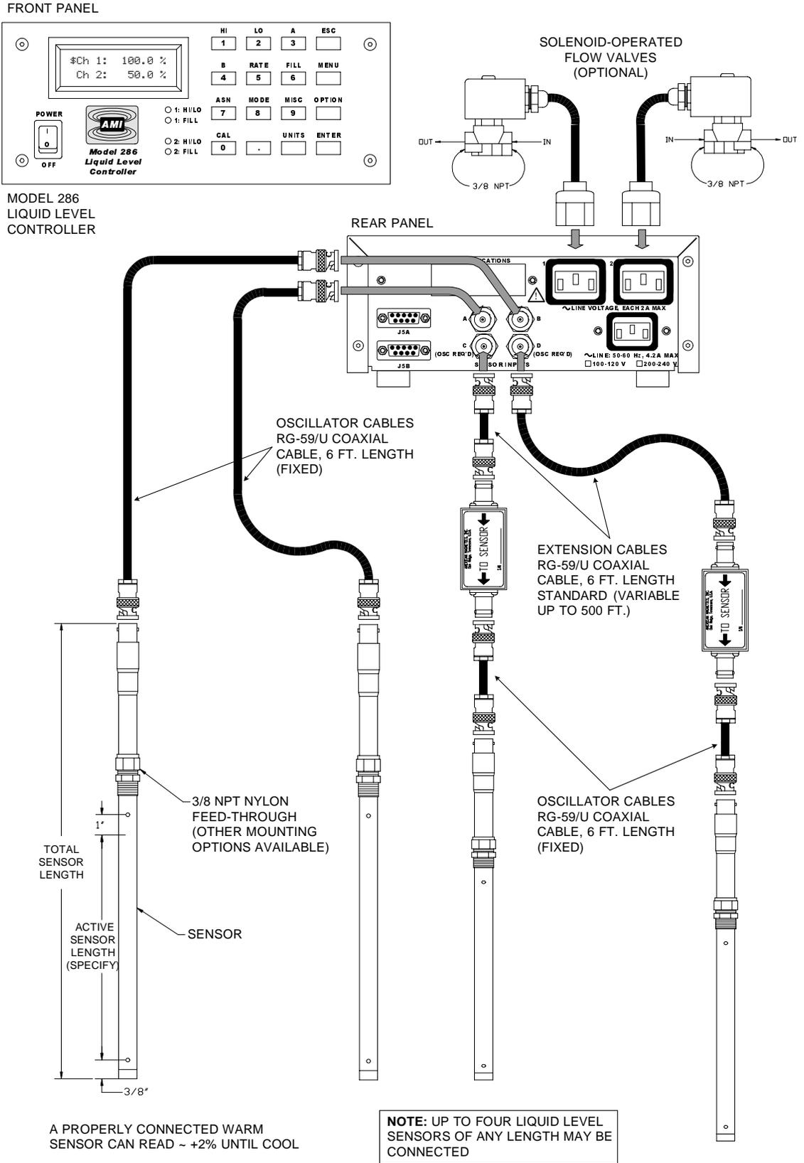
Figure 1-1. Model 286 instrument, fill valves, and sensor system diagram.
