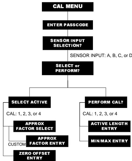
It is the responsibility of the end user to maintain accurate records of the sensor inputs and calibrations. For maximum accuracy, the various connecting components such as the cables, oscillator, and sensor should be considered a matched set. The oscillator, oscillator cable length, and sensor represent the most significant sources of variability and must be matched for a specific calibration.
