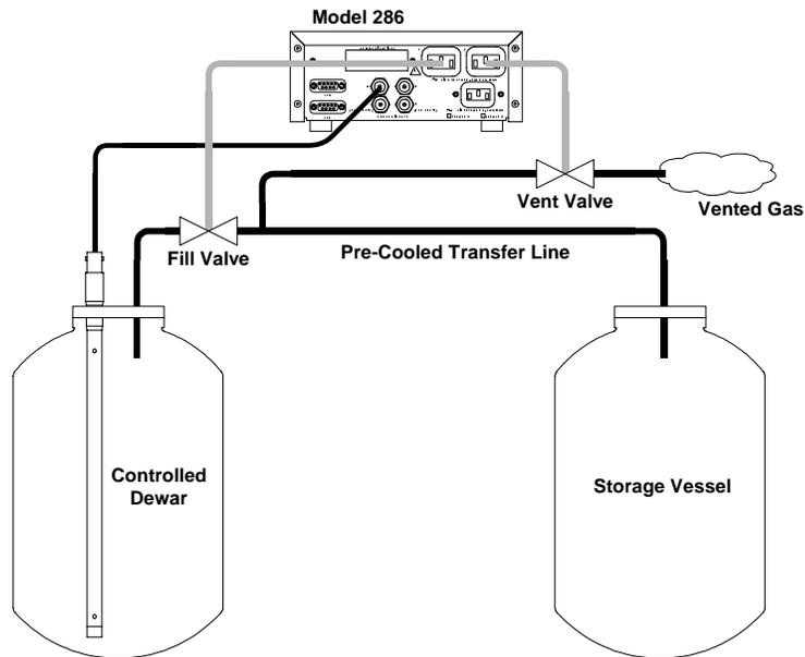
Figure 1-4. Pre-cool mode diagram illustrating one storage vessel, a vent valve, and one controlled dewar.
