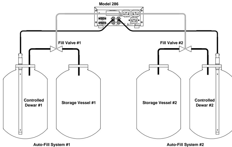
Figure 1-2. Normal mode diagram illustrating two independent auto-fill systems.
