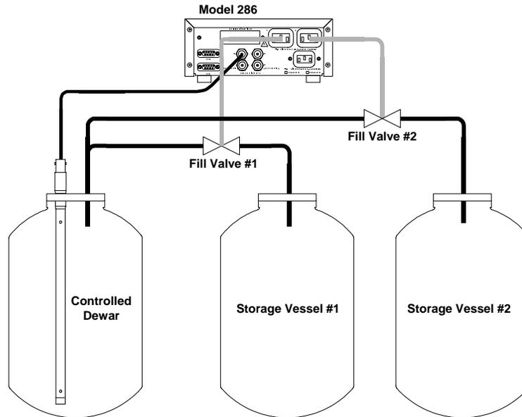
Figure 1-3. Auto-changeover mode diagram illustrating the two storage vessels and one controlled dewar.
