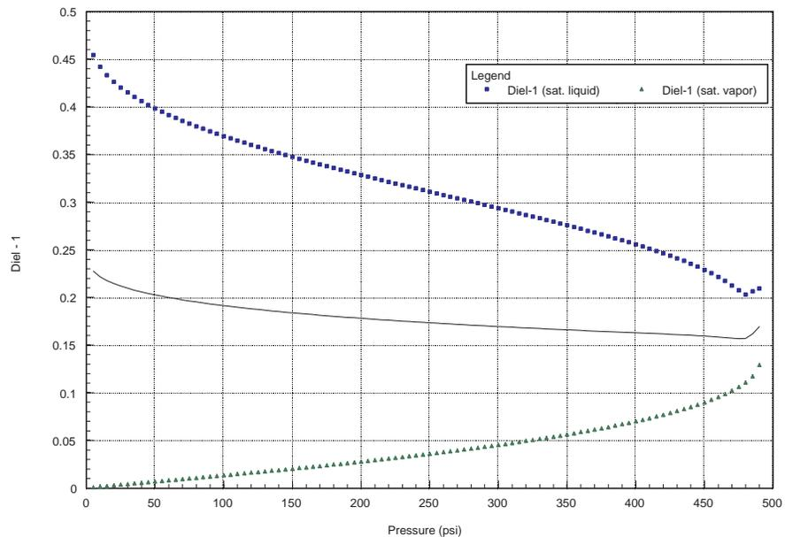
Figure 2-1. Dielectric vs. pressure for nitrogen under saturated conditions.
