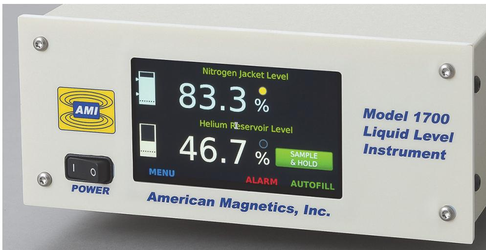
Model 1700 Front View; Dual Channel Instrument Shown
