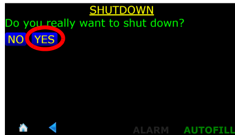
Figure 3-43. Confirming Instrument Shut Down
