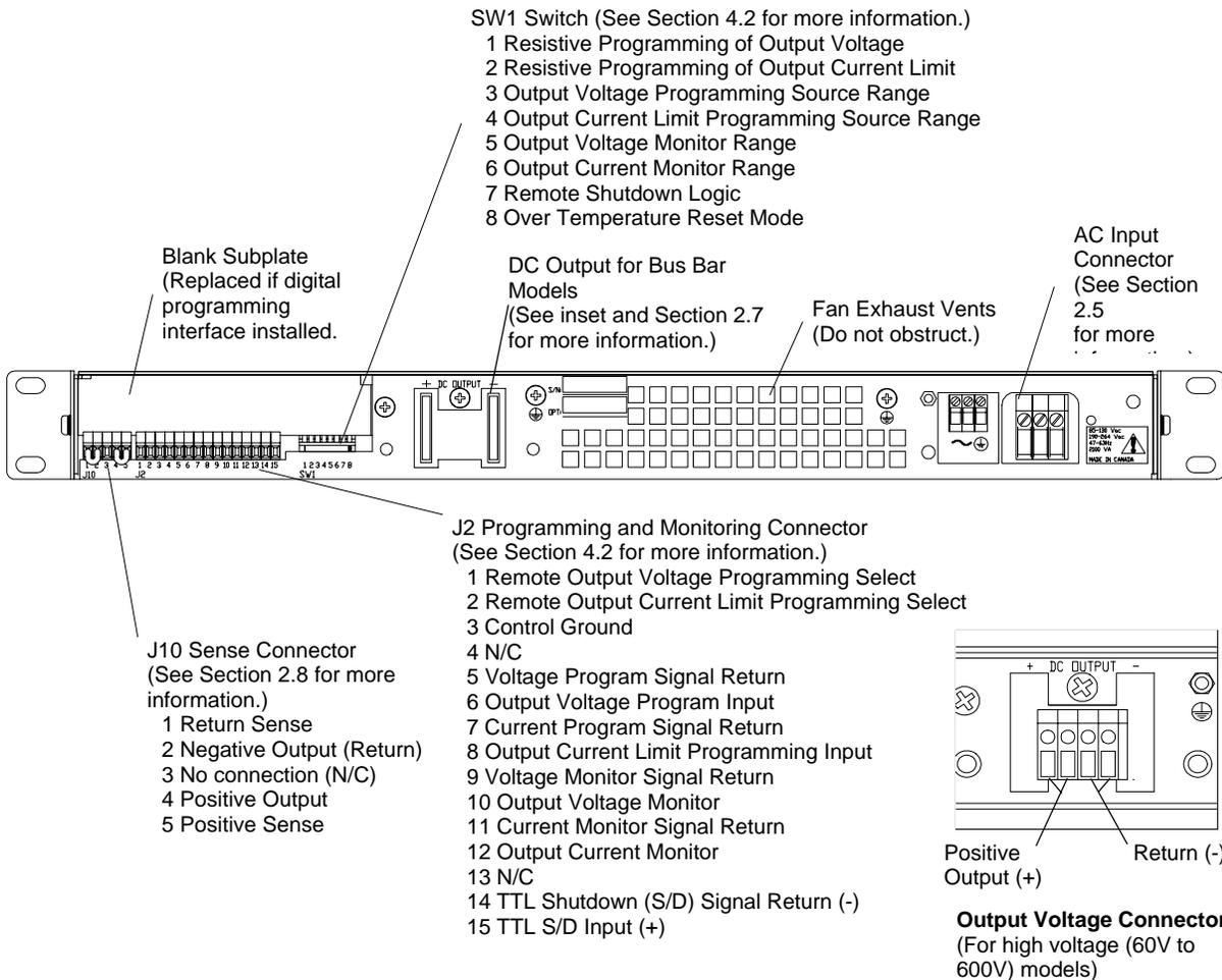
**Figure 2.3-2 Power Supply Rear Panel**
