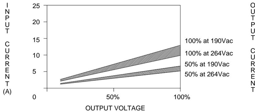
**Figure 1.3-2 Typical Input Current Characteristics, 190-264Vac Range**
