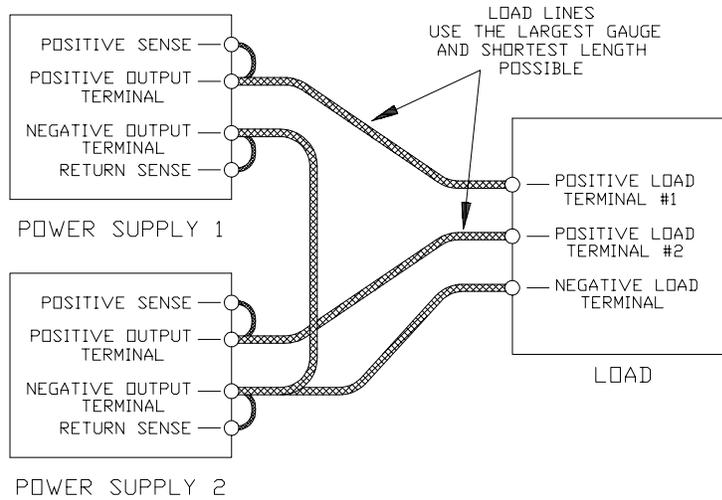
**Figure 3.5-3 Split Supply Operation of Multiple Supplies (Two Positive Voltages)**
