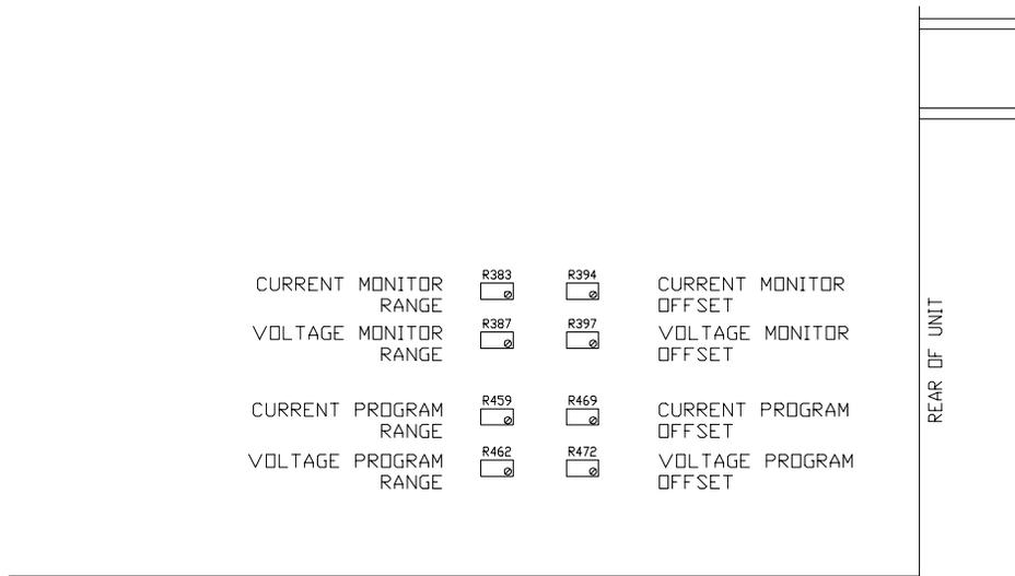
**Figure 5.2-1 Programming and Monitoring Calibration Locations
