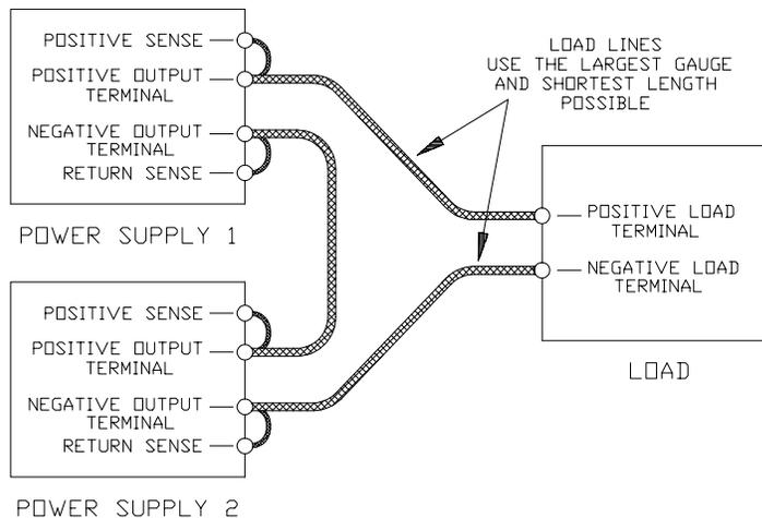
**Figure 3.5-1 Series Operation of Multiple Supplies**
