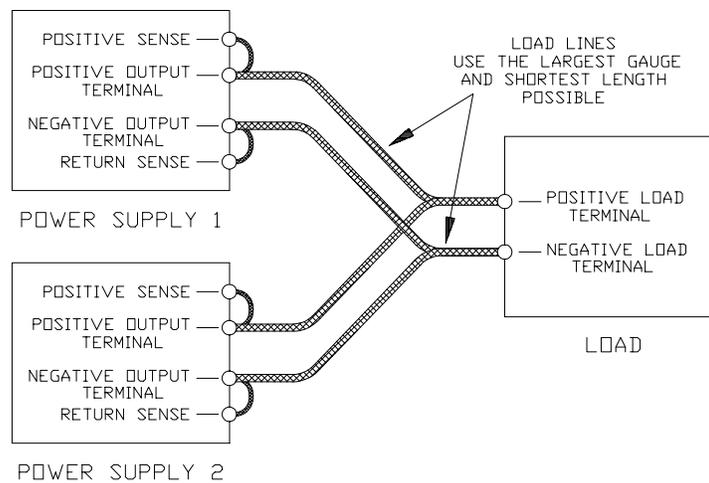
**Figure 3.5-2 Parallel Operation of Multiple Supplies**
