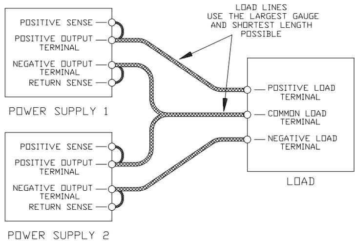
**Figure 3.5-4 Split Supply Operation of Multiple Supplies (Positive-negative Supply)**
