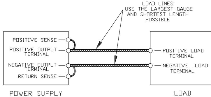
**Figure 2.7-5 Single Load with Local Sensing (Default)**
