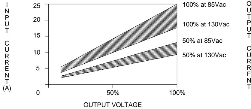
**Figure 1.3-1 Typical Input Current Characteristics, 85-130Vac Range**
