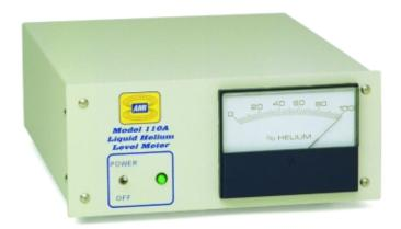
This rugged economical design is a classic. With a quick 'flip of the switch' a user can easily determine the level of liquid helium in their dewar. A large analog display clearly shows the level from 0-100% and is easily read from a distance. The Model 110 can be used with any AMI liquid helium level sensor up to 60" and comes with a standard 0-10 V recorder output on the rear panel.
