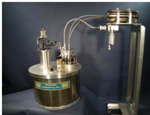
Low vibration VFVT system with remote motor option
