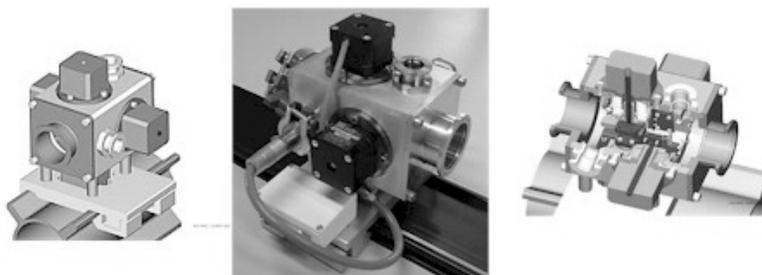
**FIGURE.6** *XMaS* in-vacuum slit system
