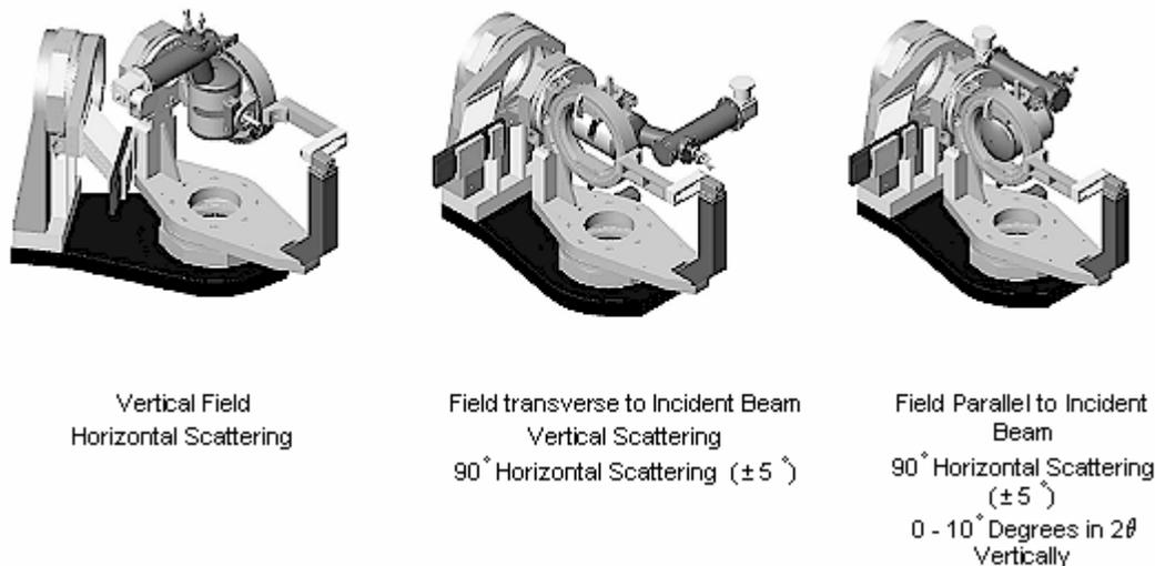
**FIGURE 1.** The *XMaS/AMI* superconducting magnet mounted within the Euler cradle on the Huber diffractometer, illustrating the three possible scattering geometries.
