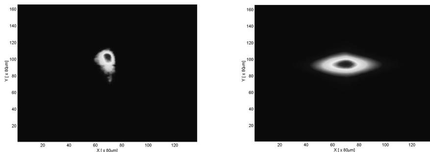
**FIGURE 3** Two images of the scattering measured at the reciprocal lattice position (0, 0, 3.385) for the Au(111) surface. The image to the left shows scattering from the Au (111) surface crystal truncation rod and the image to the right shows the effects of the copper deposition.
