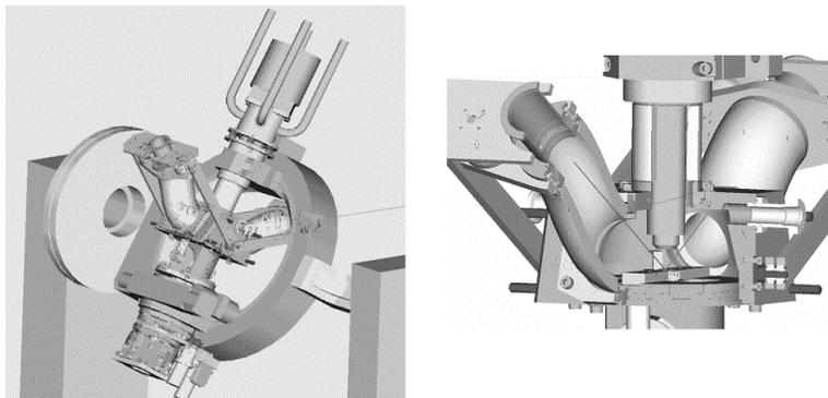
**FIGURE 5** Schematic diagrams of the in-vacuum magnet-cryostat. The beam path and magnet pole pieces can be clearly seen in the figure to the right.
