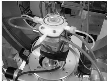
**FIGURE 2** Peltier cooled electrochemical cell mounted onto the *XMaS* diffractometer
